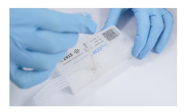
Single pipetting step – loading 300  $\mu$ L
